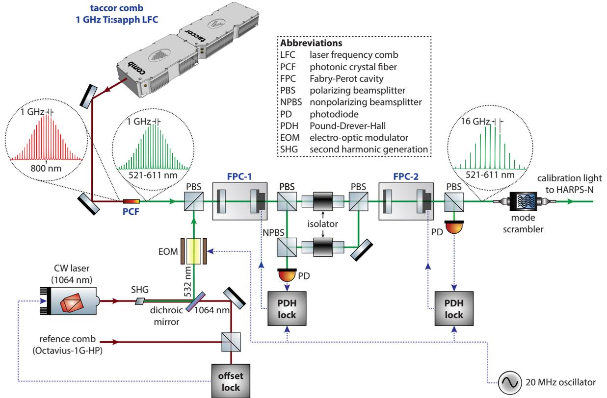
**Fig 1** Astro-comb block diagram showing a turn-key laser frequency comb that generates 1 GHz-spaced comb teeth about a center wavelength of 800 nm, a commercial photonic crystal fiber that coherently shifts the light into the visible wavelength range, and custom-built Fabry-Perot cavities that suppress 15 out of every 16 lines so as to match the resolution of the astrophysical spectrograph to be calibrated. (Abbreviations defined in figure; see text for more details.)
