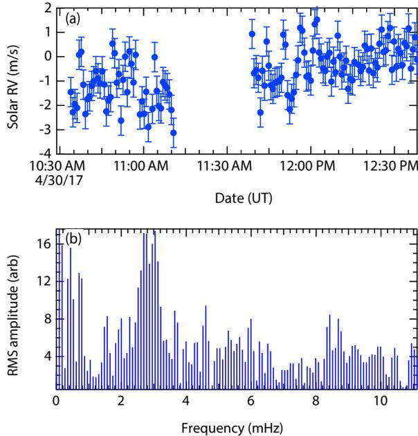
**Fig 4** (a) Comb-referenced solar RV observations. (b) Power spectrum of the data.
