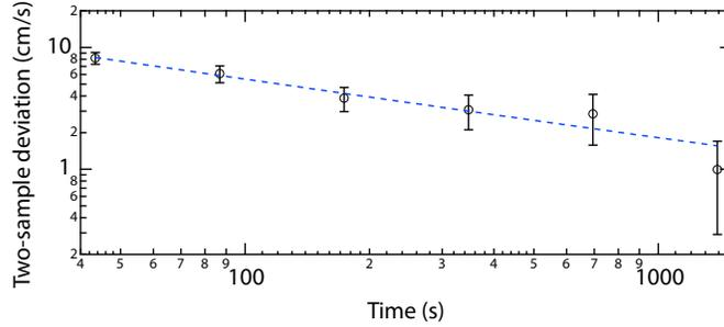
**Fig 3** Two-sample deviation of the measured frequency stability (in radial velocity units) of the astro-comb vs. averaging time. The black circles are the measured stability and dashed line is a fit consistent with the photon (shot) noise floor. The overall duration of the measurements was approximately 1 hour.
