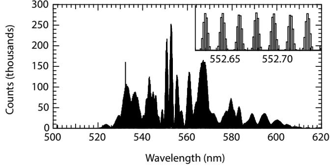
**Fig 2** Astro-comb spectrum measured with HARPS-N spectrograph. The strong peak at 532 nm is the CW reference laser used to stabilize the filter cavity lengths. (Inset) At higher spectral resolution, individual comb teeth (spectral lines) are observed.
