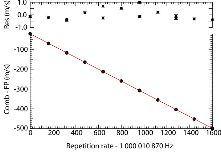
**Fig 5** Measured mean difference in astro-comb spectral lines relative to a white light FP spectrum (black circles) as a function of comb repetition rate, with a linear fit (red line), and residuals (top trace). The error bars of the residuals plot are the statistical uncertainty of  $\approx 10$  cm/s (see text).
