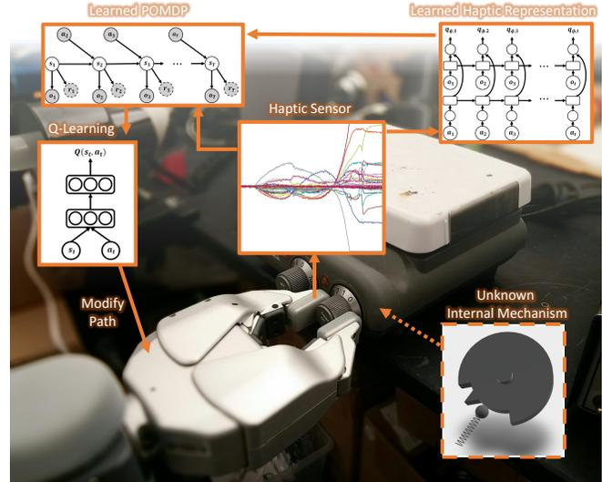
Fig. 1: **Haptic feedback** from a tactile sensor being used to modify a nominal plan of manipulation. Our framework learns an appropriate representation (embedding space) which in turn is used to learn to find optimal control.
