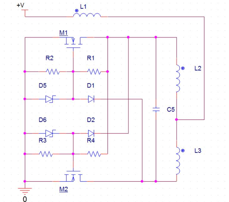
Figure 2: Schematic of ZVS driver
