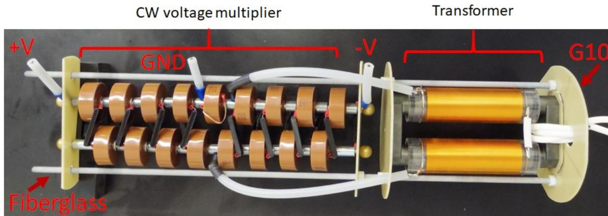
Figure 6: Assembled form. (Step-up transformer and dual voltage multiplier.)
