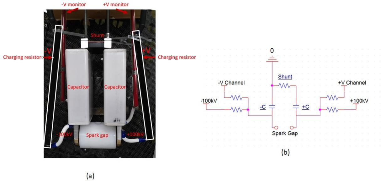
Figure 7: Brick testing station. (a) Photo of brick testing station. Charging resistors are outlined in white boxes. (b) circuit schematic
