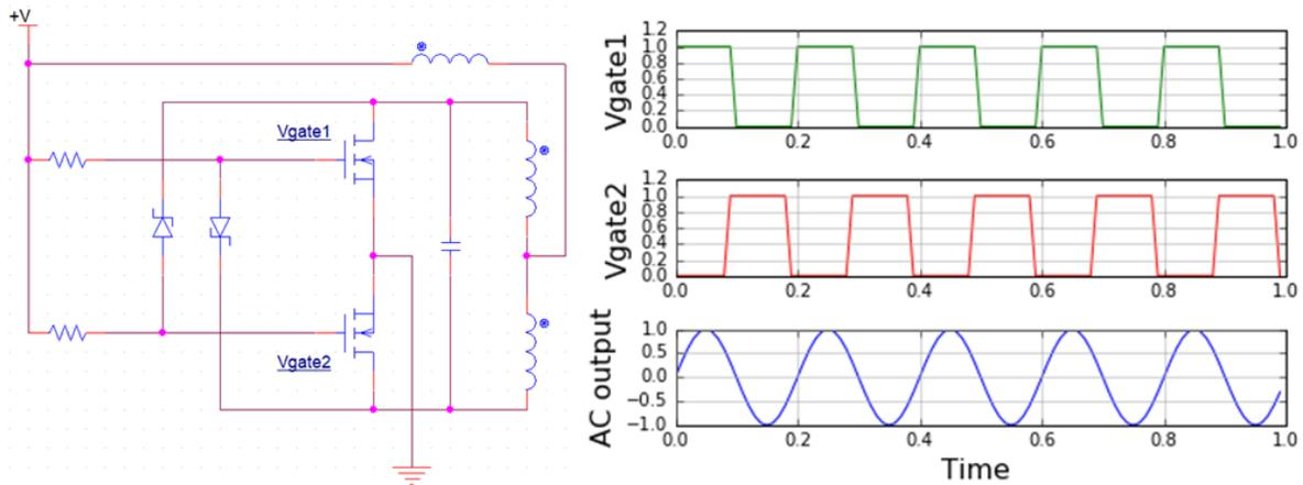
Figure 3: ZVS operating principle.
