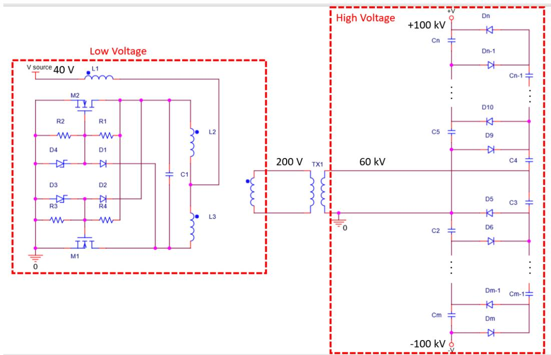
Figure 1: Circuit schematic of dual high-voltage and frequency charging system
