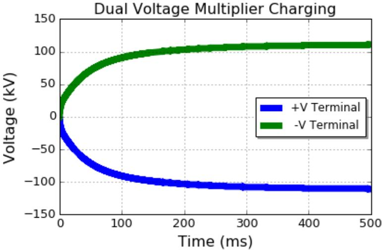
Figure 5: PSpice Simulation: Voltage vs time plot of a dual voltage multiplier charging system
