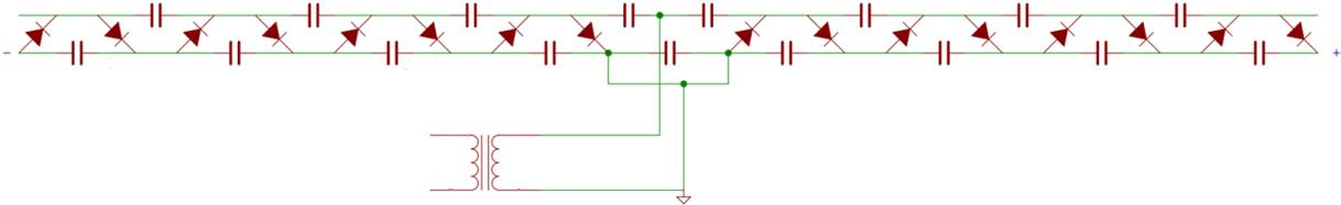
Figure 4: Schematic of dual voltage multiplier
