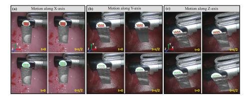
**Fig. 2.** Qualitative results of ultrasound stabilisation. The top and bottom rows are the trials without and with motion compensation, respectively. Three motion profiles were tested on a phantom (a) and *ex vivo* tissue (b-c), with directions along the X-, Y- and Z-axis of the motorised device.
