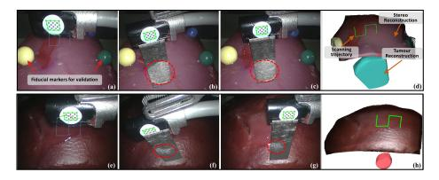
**Fig. 4.** Qualitative results of two example autonomous scanning tasks on a phantom (a-d) and *ex vivo* tissue (e-h). The obtained tumours and 3D tissue surfaces are visualised in (d) and (h). See supplementary videos for details.
