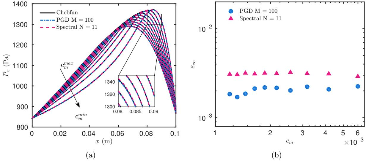
**Figure 9.** (a) vapor pressure profiles at  $t = 120$  h, for  $c_m \in [1.2 \cdot 10^{-3}; 6 \cdot 10^{-3}]$   $\text{kg}/\text{m}^3/\text{Pa}$ , and (b) the error in function of all values of moisture storage capacity between this interval.
