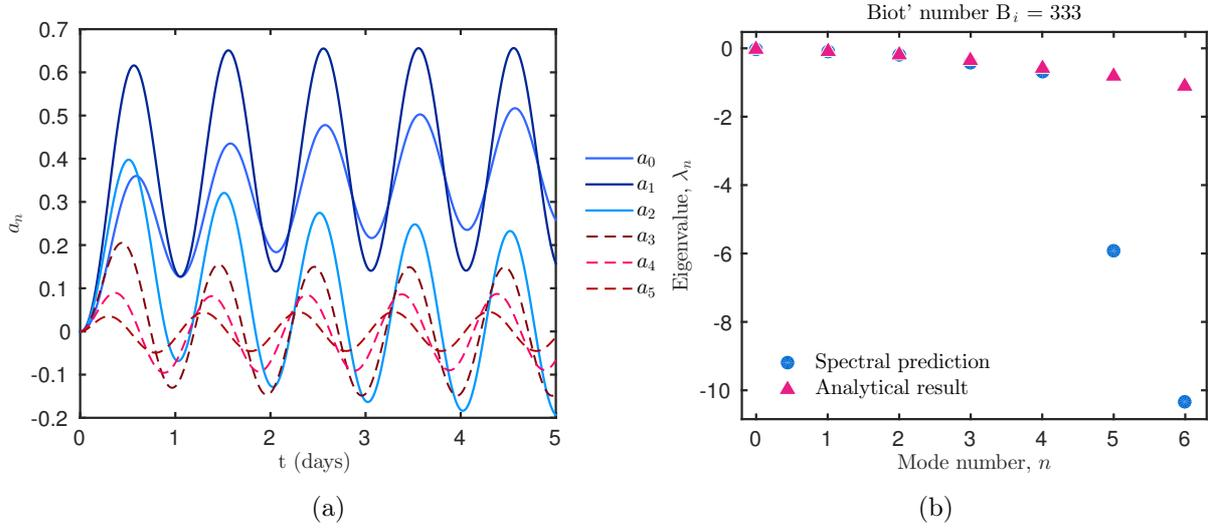
**Figure 4.** (a) Spectral coefficients as sets of time and, (b) Eigenvalues of the Analytical and of the Spectral solution corresponding to the first modes.
