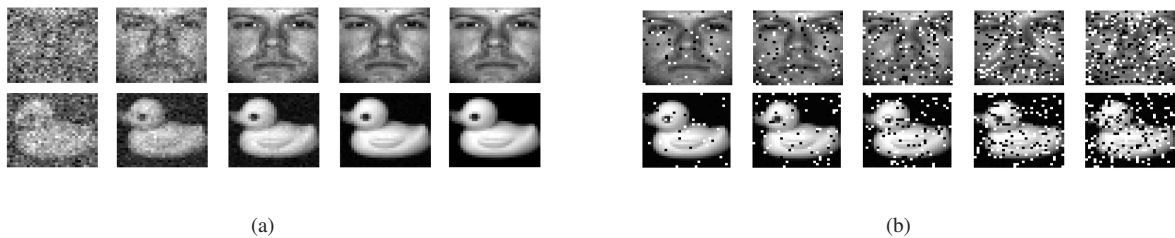
Fig. 6. (a) The corrupted samples with additive Gaussian noises under SNR equals 10, 20, 30, 40, 50 dB from left to right. (b) The corrupted samples with pepper and salt noises under the ratio of affected pixels equals 5%, 10%, 15%, 20%, 25% from left to right.
