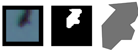
Figure 4: Low quality source image, mask, and 12-vertex simplified outline. Source image native resolution is \approx 16 \times 16 pixels.
