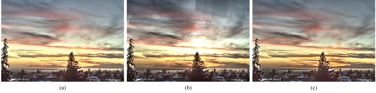
FIGURE 2: Visual comparison of HDR tone mapping. Results of (a) WLS [6], (b) FGS [20] and (c) our SG-WLS with r = 1, \tau = 1 . Blocky artifacts are noticeable in (b).
