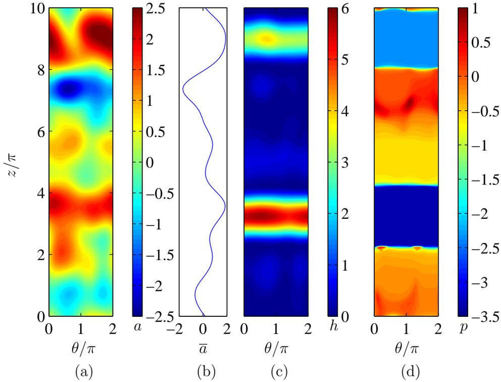
FIG. 2. A simulation from initial condition  $h = 1$  of the spatially two-dimensional evolution equation (II.1) for  $\tau = 0$ ,  $\eta = 0.5$ ,  $L = 10\pi$ ,  $r_1 = r_2 = 2$  showing the formation of equilibrium collars: (a) a realisation of the doubly-periodic wall roughness  $a(\theta, z)$ ; (b) its azimuthal average  $\bar{a}(z)$ ; (c) the near-equilibrium film thickness  $h(\theta, z, 1000)$ ; (d) the pressure  $p(\theta, z, 1000)$ .
