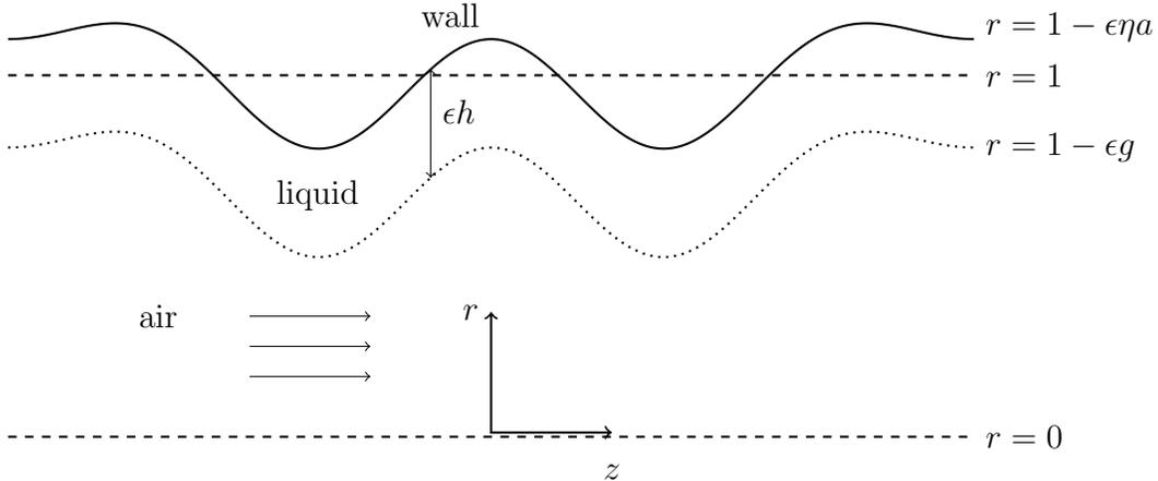
FIG. 1. A sketch of the problem domain showing axial  $a_0z$  and radial coordinates  $a_0r$  at fixed azimuthal angle  $\theta$ , showing wall location  $r = 1 - \epsilon\eta a(\theta, z)$  (solid), film thickness  $\epsilon h(\theta, z, t)$  and interface location  $r = 1 - \epsilon g(\theta, z)$  (dotted). The dashed line represents the tube centreline. The wall shape is arbitrary in this illustration.
