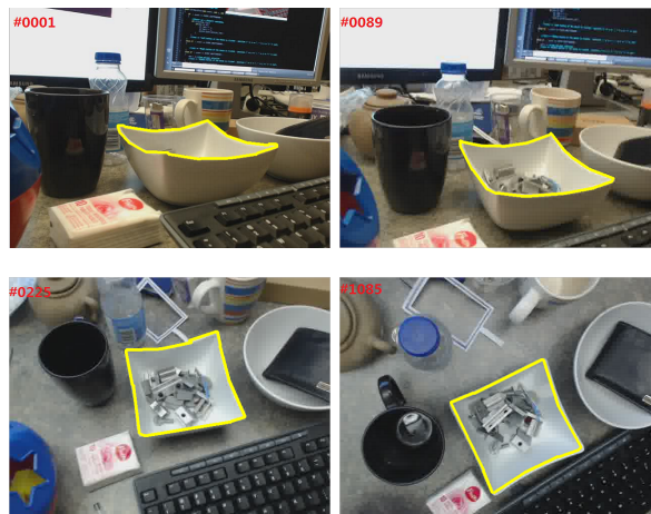
Fig. 1. Tracking the rim boundary of a bowl with the following characteristics: (1) the rim of the bowl is non-planar, (2) the bowl itself has no salient stable textures, (3) the viewpoint changes dramatically.
