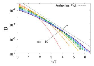
FIG. 2. Temperature dependence of the diffusion constants is shown. As the dimension is increased, super-Arrhenius behavior gets weaker.
