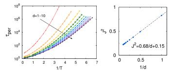
FIG. 1. (a) Temperature dependence of the mean persistence time. In all dimensions,  $\tau_{\rm per}$  is well fitted to the Eq. 3, which means the system is super-Arrhenius for all d. (b) The fitting shows that  $J^2$  is inversely proportional to the dimension, where  $J^2$  is a fitting parameter in the Eq. 3.
