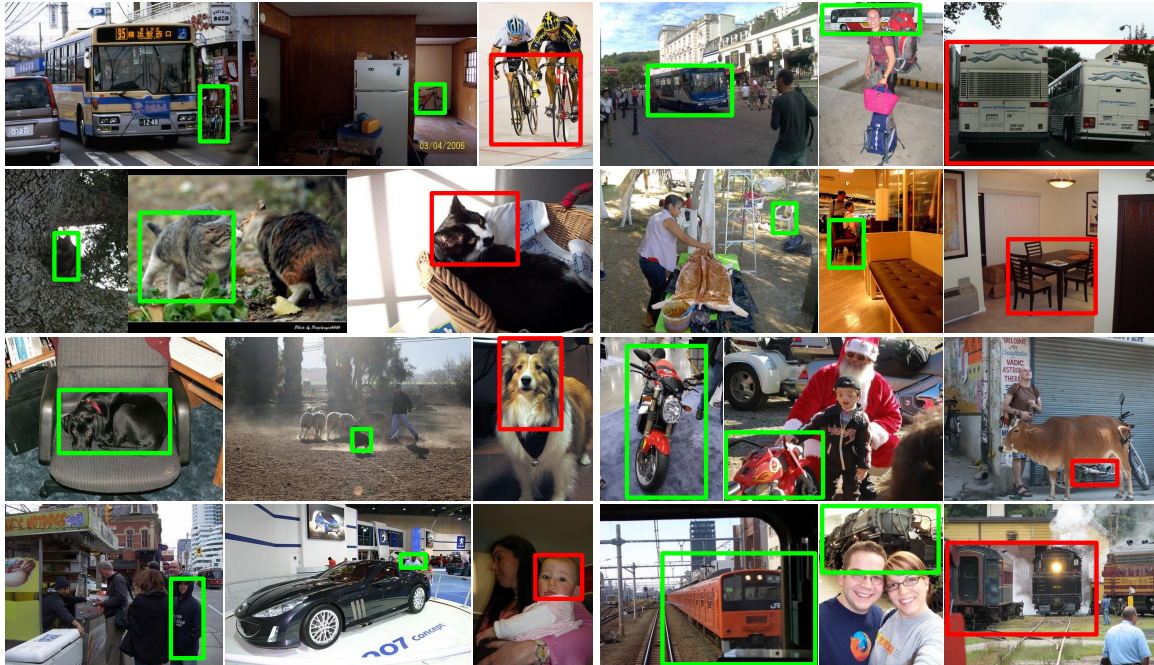
Figure 6. Some detection results for class bicycle, bus, cat, chair, dog, motorbike, person, and train. Green rectangle indicates success cases ( \text{IoU} > 0.5 ), and red rectangle indicates failure cases ( \text{IoU} < 0.5 ).
