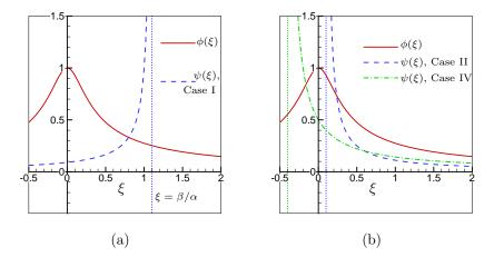
Figure 2: An auxiliary figure for the analysis below Eqs. (22) and (23). In figure (a),  $\alpha = 1$  and  $\beta = 1.1$  is used for Case I. In figure (b),  $\alpha = 5$  and  $\beta = 0.5$  is used for Case II and  $\alpha = -5$  and  $\beta = 2$  is used for Case IV. The vertical dotted lines show the asymptotic lines  $\xi = \beta/\alpha$  for each case.
