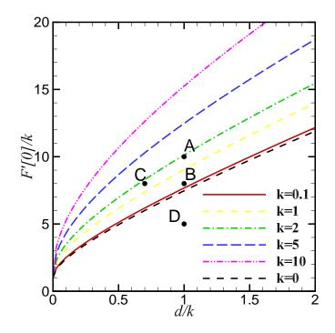
Figure 1: The diagram of the kinetic instability obtained by Eq. (7). The linear instability takes place when the stiffness of the response function F'[0]/k exceeds the critical line of each k. The numerical simulations are performed for the marks A, B, C, and D with several values of k. See Table 1.
