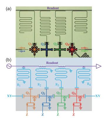
FIG. 1: (a) False color photomicrograph and (b) simplified circuit schematic of the superconducting quantum circuit for solving  $2\times 2$  linear equations. Shown are the four Xmon qubits, marked from  $Q_1$  to  $Q_4$ , and their corresponding readout resonators, marked from  $R_1$  to  $R_4$ .
