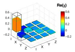
FIG. 4: Non-trace-preserving QPT characterizing the quantum linear solver. Shown are the real parts of the experimental  $\chi_{\rm exp}$  matrix (bars with color) and the ideal  $\chi_{\rm id}$  matrix (black frames), where I is the identity and  $\{X,Y,Z\}$  are the Pauli operators  $\{\sigma_x,\sigma_y,\sigma_z\}$ . All imaginary components (data not shown) of  $\chi_{\rm exp}$  are measured to be no higher than 0.015 in magnitude.
