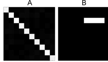
Fig. 1. The two covariance matrices generated by autoregressive process (16). A)  $C(0)$ , the covariance matrix with support at zero lag; B)  $C(20)$ , the covariance matrix at lag  $\tau = 20$ . This matrix is identical to that at  $\tau = 40$  and  $\tau = 60$ .
