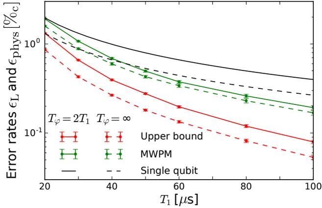
FIG. 4.  $T_1$  dependence of the Surface-17 logical error rate (MWPM and UB) and the physical error rate. We either fix  $T_\phi = 2T_1$  (solid) or  $T_\phi = \infty$  (dashed). Logical error rates are extracted from a best fit of Eq. (2) to  $\mathcal{F}_L[k]$  over  $k = 1, \dots, 20$  QEC cycles, averaged over  $N = 50,000$  runs. Error bars (2 s.d.) are calculated by bootstrapping.
