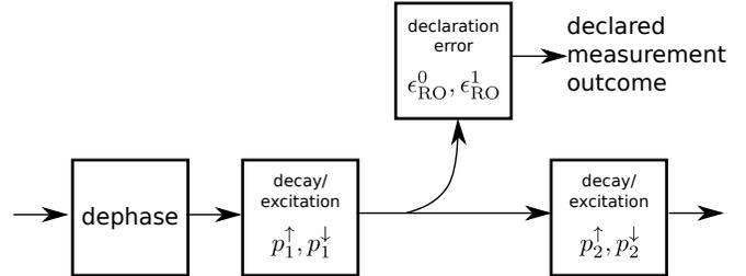
FIG. 9. The model for measurements consists of a dephasing of the qubit followed by a period of decay and excitation with probability  $p_{\downarrow/\uparrow}^{(1)}$ . At this point, the qubit state is sampled. The sampling result is subject to a declaration error  $\epsilon_{RO}$ , and the qubit state is subject to further decay or excitation with probabilities  $p_{\downarrow/\uparrow}^{(2)}$  before the end of the measurement block.
