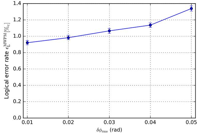
FIG. 11. Logical error rate for Surface-17 as a function of two-qubit phase error, using the MWPM decoder. Other parameters are as given in the main text.
