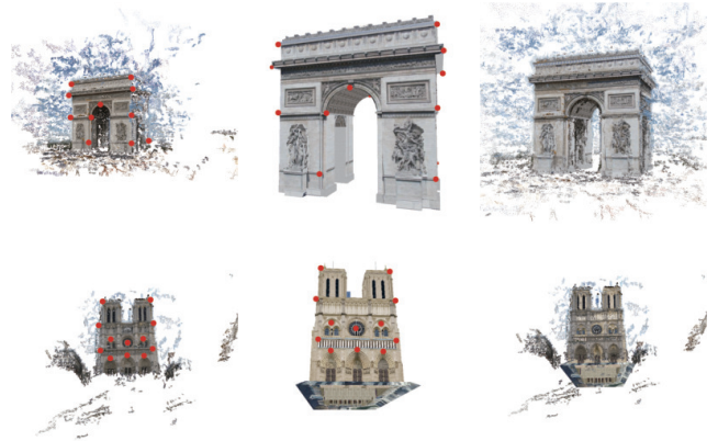
Fig. 2: Registration between the point cloud model (left) and mesh model (middle) based on the marked points (red). We align the mesh model with the point cloud model using the registration parameters. The transformed mesh model coincides with the point cloud model (right).
