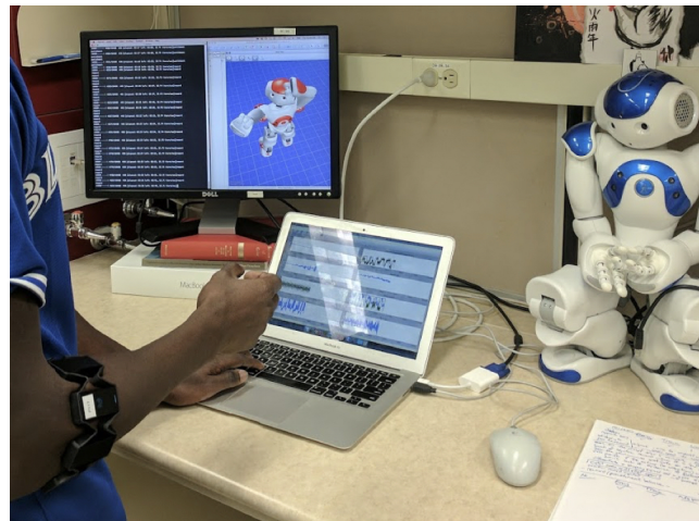
Figure 1. Experimental configuration. One of the study participants with the Myo band on their right arm providing a control signal, while simultaneously providing feedback signals with their left hand. The Aldebaran Nao robot simulation is visible on the screen alongside experimental logging.
