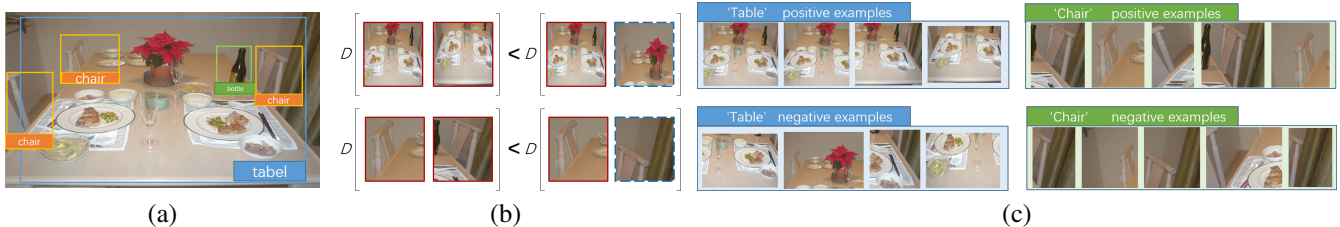
Fig. 2. Object detection is based on the classification of RoIs (proposals). The triplet embedding works on the groundtruth of object ROIs (a), the positive and negative ROIs (c) with respect to different object classes (like Table and Chair), in which the similarity distance constraint (b) is applied.
