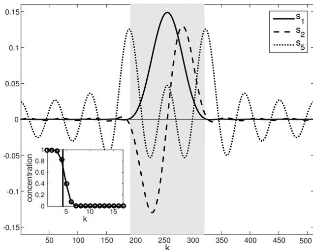
Fig. 1. Example of 1-D Slepian vectors for a signal of length  $N = 512$ . Three example vectors are shown for the selected interval indicated with the gray background. The energy concentration is plotted in the inset and the Shannon number is marked by the vertical bar.
