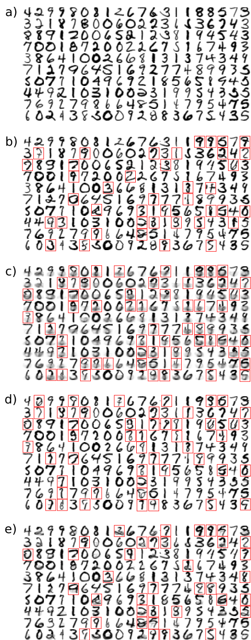
Figure 3: Test and reconstructed images from the digit completion application. Reconstructed digits were generated by concatenating the predicted responses with the upper -input- half of the test images. Bad reconstructions are enclosed in red squares. (a) Test digits. (b)-(e) Reconstructions using predictions from (b) 1NN, (c) RF, (d) kRF and (e) dRF.
