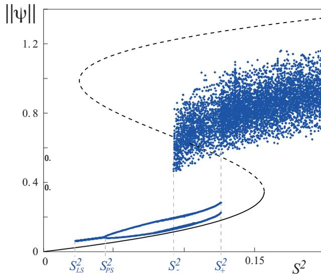
FIG. 3. (color online) Bifurcation diagram of model Eq. (1). The total intracavity intensity  $\|\psi\|$  versus the pump intensity  $S^2$  with  $\delta = 1$ , and  $\alpha = 0.16$ . The continuous and dashed thick line points out the stable and unstable HSS, respectively. The continuous blue lines indicate the extrema of the total intracavity intensity  $\|\psi\|$  of localized states. The cloud of blue scattered points accounts for the spatiotemporal chaotic state.
