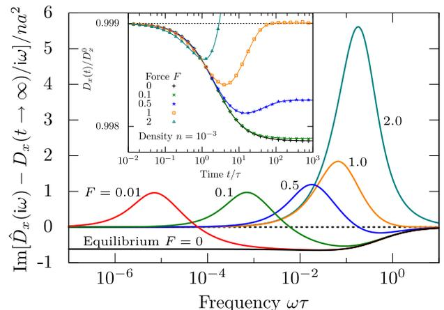
FIG. 2. Imaginary part of the frequency-dependent response encoding the approach to the stationary state for different strength  $F$  of the driving. Inset: Time-dependent diffusion coefficient for different forces exemplifying the nonmonotonic behavior. Symbols correspond to simulation results and lines represent the theory.
