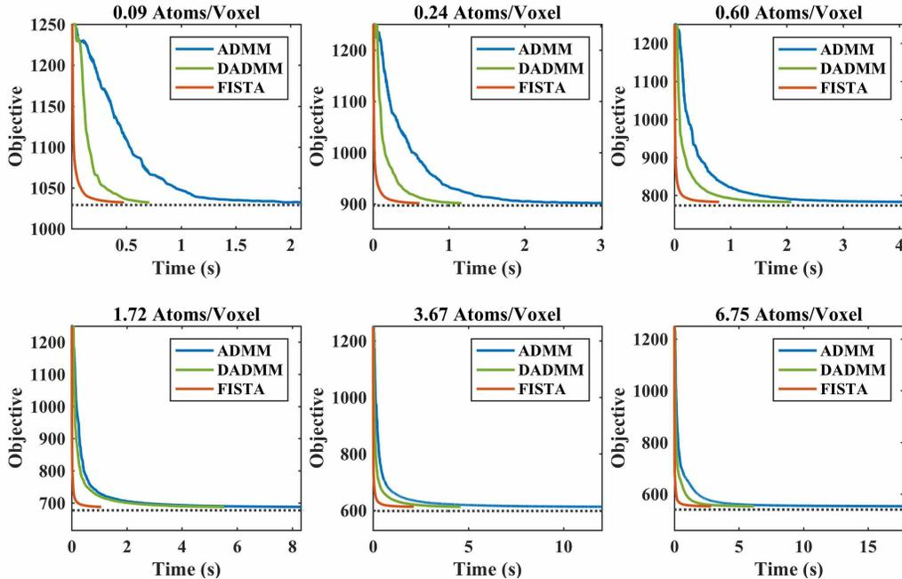
**Figure 8:** Comparison of time for completion of Kron-ADMM, Kron-DADMM, and Kron-FISTA on a 2D  $50 \times 50$  phantom HARDI data using Haar-SR for various sparsity levels. Kron-FISTA consistently reaches the minimum objective in the least amount of time. For number of iterations and lambda values, see Table 4.
