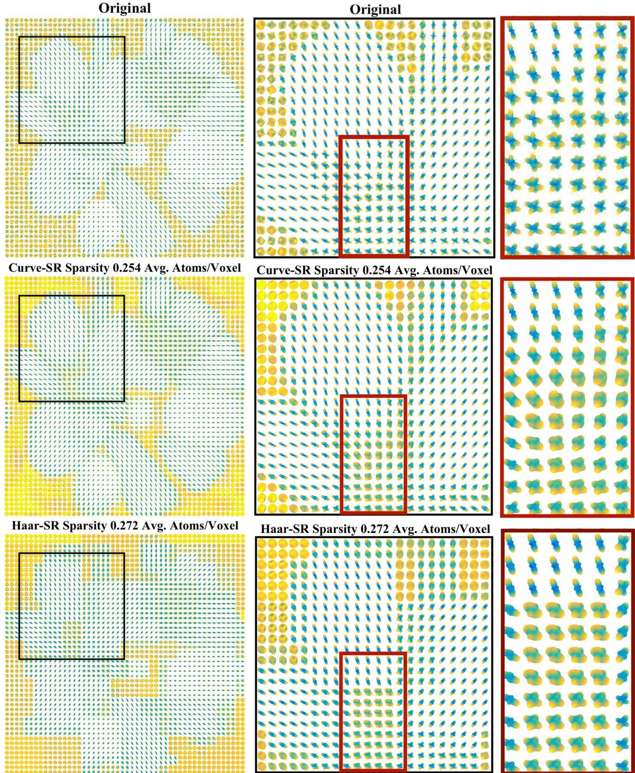
**Figure 10:** Results of the proposed spatial-angular sparse coding using Kron-FISTA for Haar-SR and Curve-SR using an average of  $\sim 0.25$  atoms/voxel compared to original signal. Curve-SR outperforms Haar-SR in this regime due to its additional directionality. We can see a drastically better reconstruction compared to the state-of-the-art at the same sparsity level in the top left of Figure 2. This clearly shows that we can achieve accurate reconstruction with less than 1 atom/voxel.
