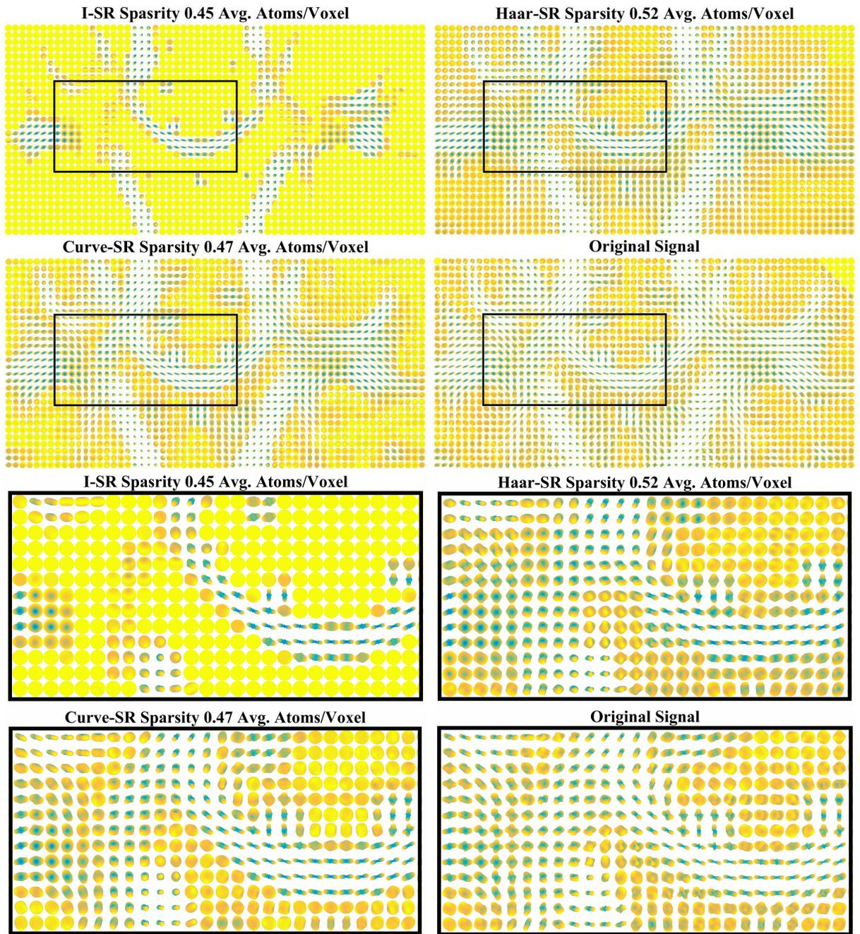
**Figure 13:** Results of proposed spatial-angular sparse coding on real HARDI brain data using Kron-FISTA for I-SR, Haar-SR and Curve-SR using an average of  $\sim 0.5$  atoms/voxel compared to original signal. Curve-SR outperforms Haar-SR in this sparsity range due to its directionality. The state-of-the-art I-SR is unable to compete at this sparsity level.
