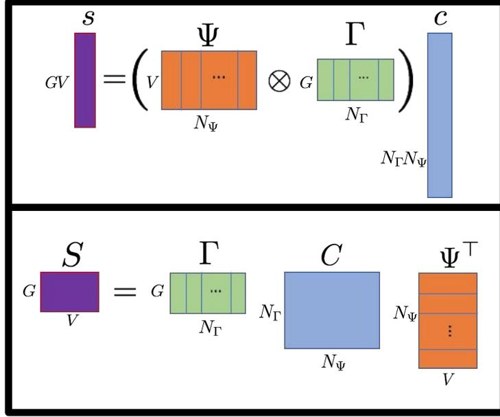
**Figure 6:** Equivalent vector form (top) and matrix form (bottom) for the Kronecker decomposition of a signal. We propose to use the matrix form which provides a more compact representation for signals of large size and exploits the full separability of the Kronecker product, reducing matrix multiplication complexity from  $O(GVN_\Gamma N_\Psi)$  to  $O(GVN_\Gamma)$ .
