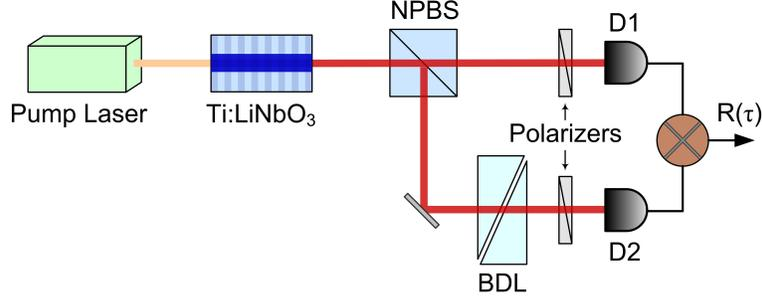
Figure 2: Schematic of the quantum interferometer based on hyper-entangled states generated in type-II down conversion.
