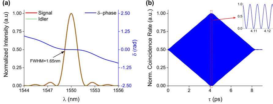
Figure 3: Spectral parameters and quantum interference of SPDC radiation obtained in a uniformly poled 16.5 mm long sample. (a) perfectly overlapping signal and idler spectral intensity and spectral phase  $\delta$  coefficient distribution; (b) the intensity correlation interferogram.
