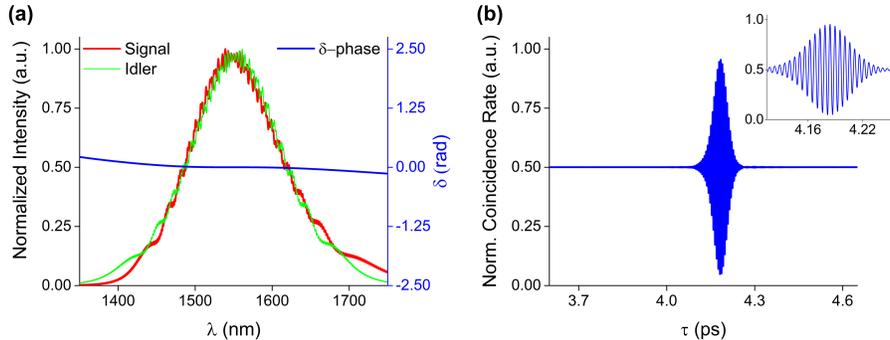
Figure 7: The SPDC spectrum, phase  $\delta$ , and the optimized interferogram produced using asymmetric poling Eq.(15) in case of  $N = 11$ . The spectral width of the intensity envelope (FWHM) is 135 nm.
