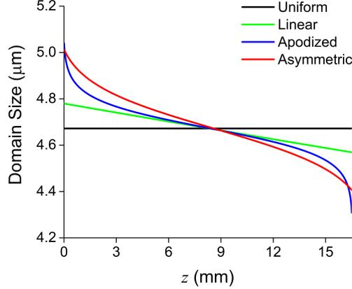
Figure 6: Different poling profiles along the length of nonlinear crystal interaction region  $z$ .
