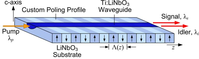
Figure 1: Schematic of the type-II SPDC source based on periodically poled Ti:PPLN waveguide.
