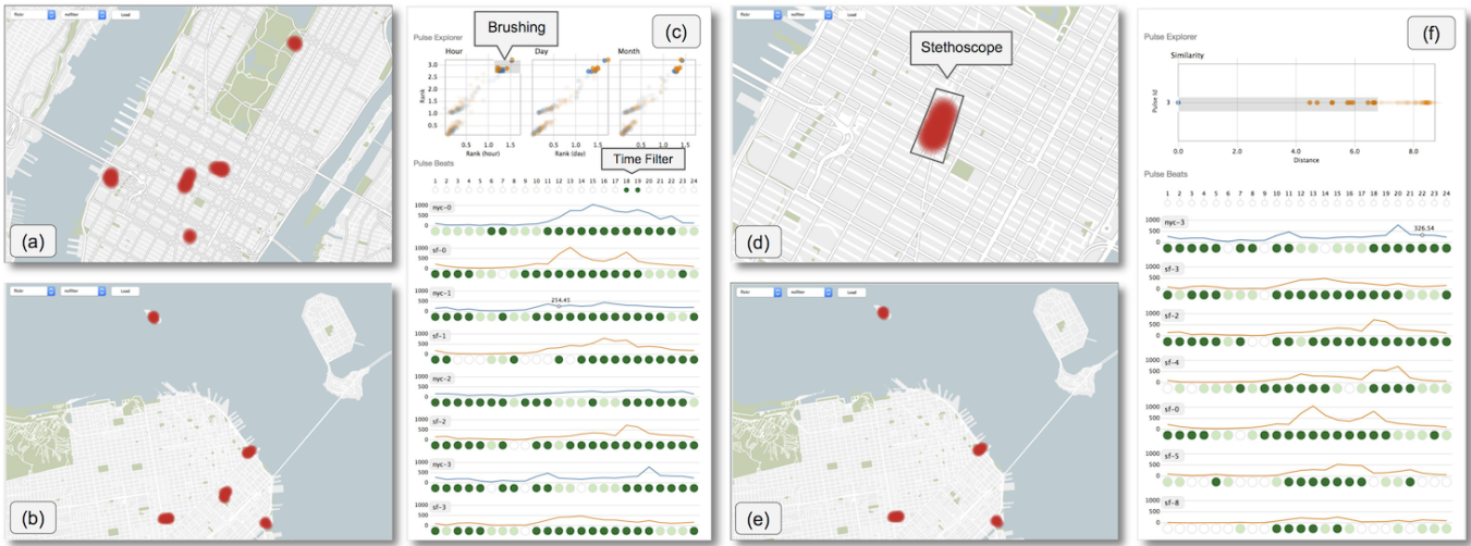
Fig. 6. Visual Exploration Interface of the Urban Pulse framework. (a), (b) show two map instances highlighting the highest ranked pulses at the hour resolution. These pulses are selected by brushing the scatter plot in the pulse monitor, shown in (c). The pulse monitor also visualizes the beats of currently selected pulses. The different colors of the points in the scatter plot, as well as the beats viewer, correspond to the different map widgets (blue for NYC and orange for SF). The shown beats can be filtered using the time filter. The Stethoscope tool is used to select the pulse corresponding to Times Square in (d). It is then used to query for similar pulses in San Francisco. The scatter plot in the pulse monitor is updated to show the result of the query, shown in (f). Selecting the closest pulses using the scatter plot highlights these pulses on the map widget, see (e).
