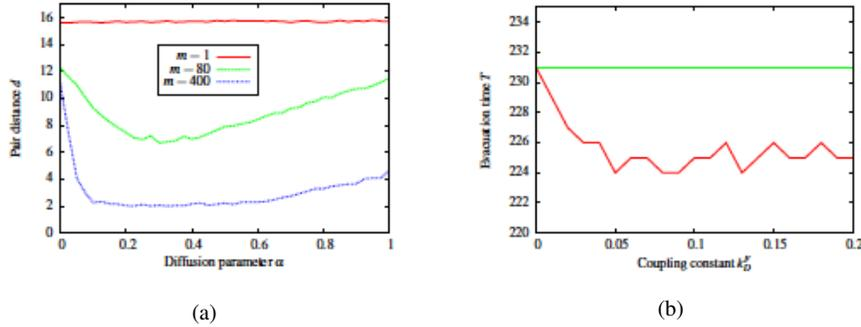
Fig. 1: Different views on the DGFF model. **(a)** Dependence of the average pair distance  $d$  on the diffusion parameter  $\alpha$  for different values of the boson multiplicity  $m$ . **(b)** Dependence of  $T$  on  $k_D^F$ . The dashed line refers to  $T = T_{hom}$ , which is the average evacuation time of a homogeneous crowd without pair bonds.
