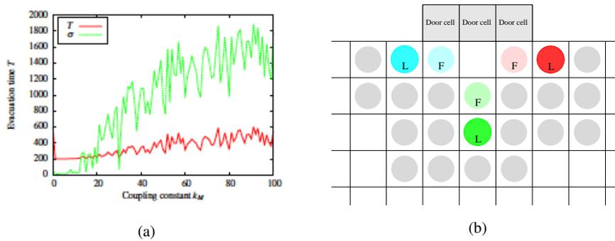
Fig. 3: Clogging in systems with MTFF. **(a)** Dependence of evacuation time  $T$  on the coupling strength  $k_M$  with  $k_S^L = 0.8$  and  $k_S^F = 0.2$ . High values of  $k_M$  lead to increased values of  $T$  and high  $\sigma(T)$  due to clogging. **(b)** Example for a typical clogging situation for a system with door width  $d = 3$ .
