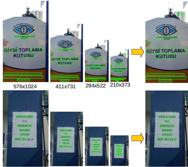
Fig. 3. Multi-scale text detection. The original image is downsized by 1.4 at each step until one side becomes less than 200 pixels. Detections at each scale are combined to obtain the final detections, shown on the right.
