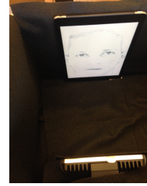
Figure 9: Our simplified physical world has a tablet with retina and a fixed webcam in a low-glare box.
