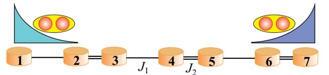
FIG. 1. Dimer lattice of nonlinear cavities with the tunneling constants  $J_1$  and  $J_2$ . Two-photon edge states are sketched.
