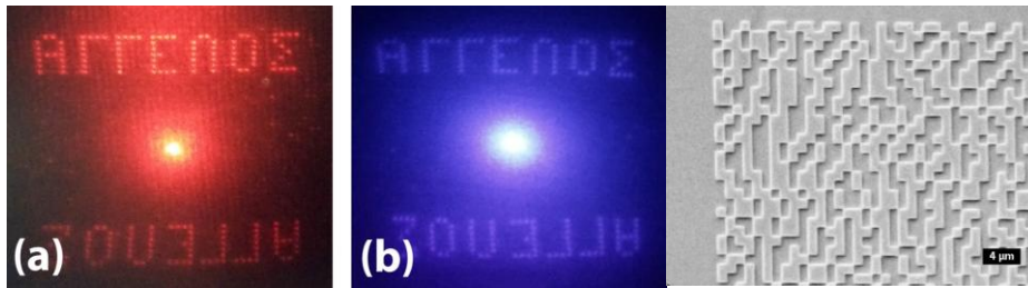
Figure 9 (left) The reconstruction of the surface relief hologram under laser illumination at (a) 650nm and (b) 404nm. (right) Scanning electron micrographs of the patterned hybrid film.
