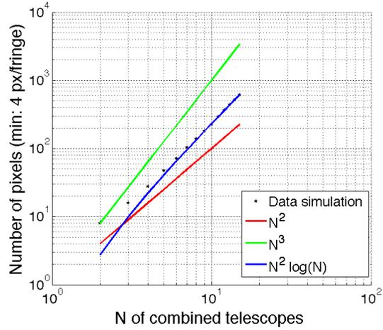
Figure 2. Left: non-redundant fiber arrays optimized for compact beam combination of up to 15 telescopes (from Lacour 2010<sup>29</sup>). Right: number of pixels per wavelength channel needed to code all the information of the baselines, as a function of the combined telescopes (stars). A minimal sampling of 4 pixels per fringe is assumed. Red line:  $N_t^2$  scaling law. Green line:  $N_t^3$  scaling law. Blue line:  $N_t^2 \log(N_t)$  scaling law.
