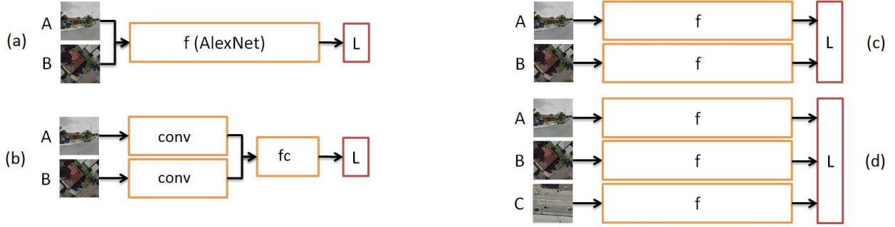
Fig. 3. Different CNN architectures: on the left is the first category: the classification network and the Siamese-classification hybrid network, on the right is the second category: the Siamese network and the triplet network
