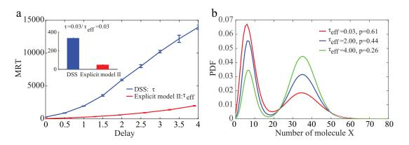
FIG. 2. a) Mean residence time calculated by the DSS and by explicit model II. Inset: Mean residence time of low number state when the delay is near zero.b) Equilibrium distribution calculated by explicit model II. Legend: p is the proportion occupied by low number state. All parameters are the same as in Fig 1.
