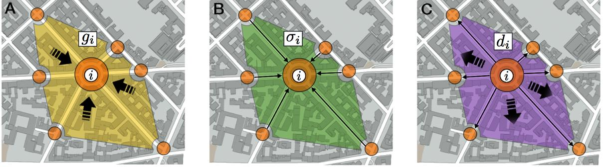
FIG. 1. Illustration of the variables of the MCM model. (A) Vehicles entering junction  $i$  from the area surrounding  $i$ . (B) Vehicles entering junction  $i$  from its neighboring junctions. (C) Vehicles leaving junction  $i$ , either to go to other neighboring junctions or to finishing the trip in its surrounding area.
