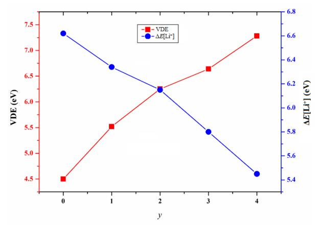
Fig. 4. The plots of VDE of  $BH_{4-y}(BH_4)_y^-$  hyperhalogen anions and  $\Delta E[Li^+]$  of  $LiBH_{4-y}(BH_4)_y$  salts as a function of *y*.
