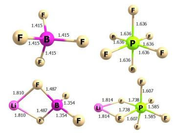
Fig. 1. Equilibrium structures of  $BF_4$ ,  $PF_6$  superhalogen anions and their Li-salts, which are currently used as electrolytic salts in LiBs. The bond lengths in Å are calculated at  $\omega B97xD/6-311+G(d)$  level.
