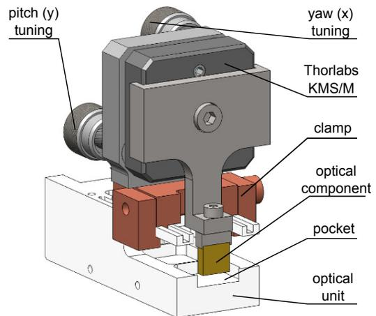
FIG. 2: Toolkit used to align component in the optical unit. The yaw and pitch angle can be adjusted independently using the two knobs. The component is aligned within a pocket that is machined into the optical unit. Epoxy is applied to secure the component within this pocket after alignment. After the epoxy has cured, the adjuster is removed enabling the compact form-factor.
