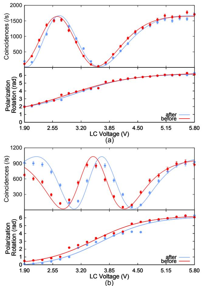
FIG. 3: Coincidence rate and calibration curve for the liquid crystal (LC) polarization analyzer for the primary (a) and secondary (b) experimental profiles. Both liquid crystals show a reduced ability to perform polarization rotation.
