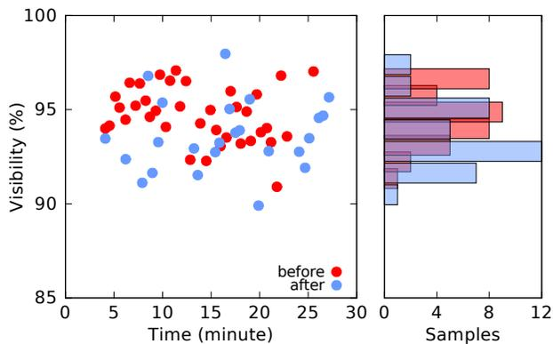
FIG. 4: Comparison of polarization visibility before (red) and after (blue) explosion for a number of experimental runs taken over 30 minutes. The average baseline visibility is  $95 \pm 1\%$  while the recovered package exhibited a visibility of  $94 \pm 2\%$ , showing no significant deviation after the explosion. The histogram on the right shows the distribution of the visibility.
