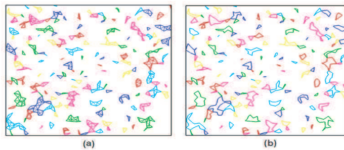
Figure 13 (Color online) Cluster structure formed from 1000 random discrete points in a two-dimensional square area [0,1] \times [0,1] . (a) A cluster; (b) the corresponding cluster boundary. (Adopted with permission from Ref. [51]. The grey-level version is published in Ref. [52].)
