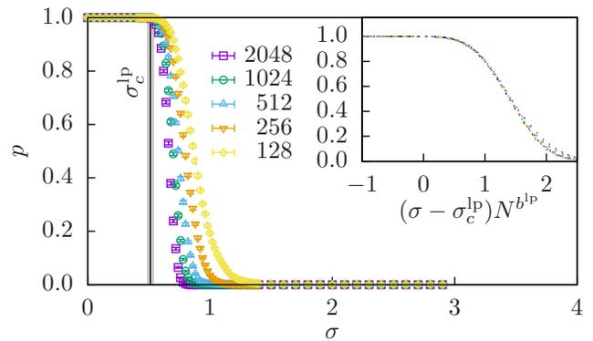
FIG. 4: (color online) Probability  $p$  that the degree LP relaxation is integer. The inset shows the collapse for  $N \geq 256$ , with  $\sigma_c^{\text{lp}} = 0.51(4)$  and  $b^{\text{lp}} = 0.29(6)$  obtained from the same type of analysis as in Fig. 3 for  $N \geq 512$ .
