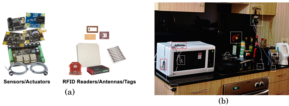
Fig. 5. (a) some sensors and RFID devices; (b) WoT-enabled microwave oven
