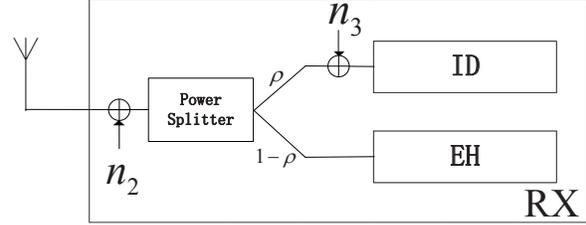
Fig. 1. An FD point-to-point system with SWIPT, where FD- Fig. 2. The receiver of FD-MS applies PS scheme to decode AP and FD-MS are equipped with  $M + N$  and two antennas, information and harvest energy simultaneously.
