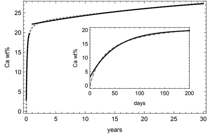
**Figure 4** – Experimental mineralisation kinetics from Ref. [47] (dashed) together with two exponential fits of the form  $m_{\text{max}} - (m_{\text{max}} - m_f) e^{-k_m t}$  (solid lines). The short-time fit has  $m_f = 3$  Ca wt%,  $m_{\text{max}} = 20.1$  Ca wt%,  $k_m = 0.0194/\text{day}$  (also shown in the inset). The long-time fit has  $m_f = 21.85$  Ca wt%,  $m_{\text{max}} = 30.4$  Ca wt%,  $k_m = 9.3 \cdot 10^{-5}/\text{day}$ .
