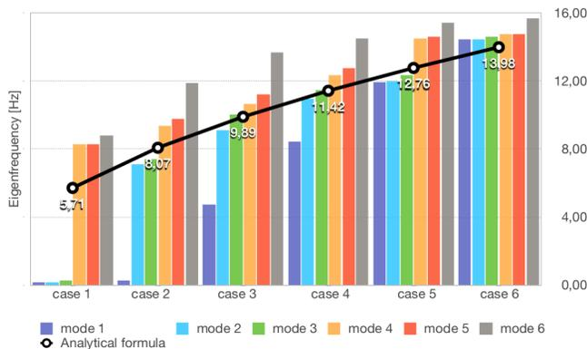
Figure 4: Asymptotic (black curve) versus numerical (color bars) results for the first six local resonances associated with iron spheres of radius  $R = 3.7$  m attached to a bulk of concrete with one (case 1) up to six (case 6) iron ligaments of length  $l_i = 0.3$  m and diameter  $h_i = 0.2$  m.
