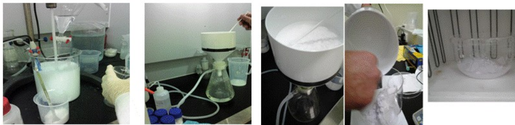
Figure 7.14: Calcium carbonate production: neutralization with liquid \text{NH}_3 (left), filtration, and purified product (right).
