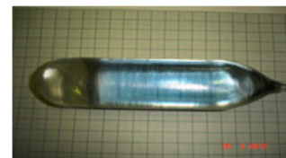
Figure 3.14: ^{48\text{depl}}\text{Ca}^{100}\text{MoO}_4 crystals grown at the Innovation Center of the Moscow Steel and Alloy Institute (ICMSAI) in Russia.
