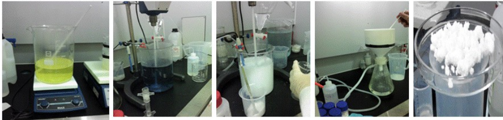
Figure 7.13: The procedure to obtain crystals of molybdate; \text{CaMoO}_4 solution (left), neutralization with liquid \text{NH}_3 , vacuum filtration, and crystals of molybdate (right).
