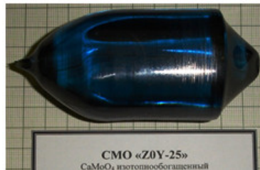
Figure 3.14: ^{48\text{depl}}\text{Ca}^{100}\text{MoO}_4 crystals grown at the Innovation Center of the Moscow Steel and Alloy Institute (ICMSAI) in Russia.
