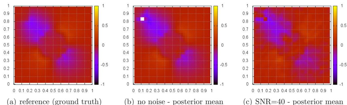
**Figure 12.** Example 2: Comparison of shear stress'  $\sigma_{xy}$  spatial distribution with the posterior means obtained when data have no noise and for SNR=40dB.
