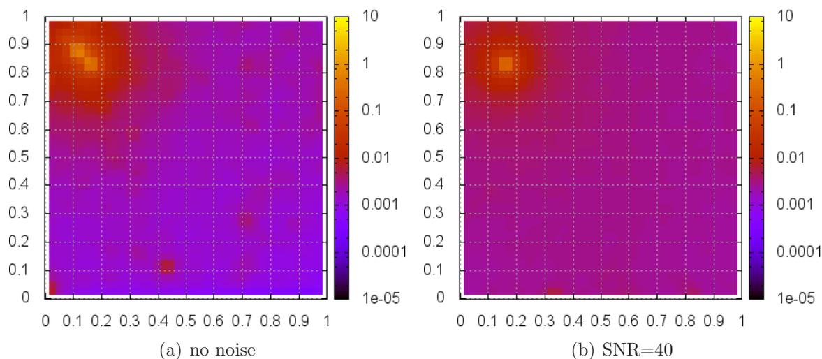
**Figure 8.** Example 2: Model discrepancies/errors  $\{\lambda_e^2\}_{e=1}^{n_{el}}$  for a) no noise, and b)  $\text{SNR}=40\text{dB}$  (in log-scale)
