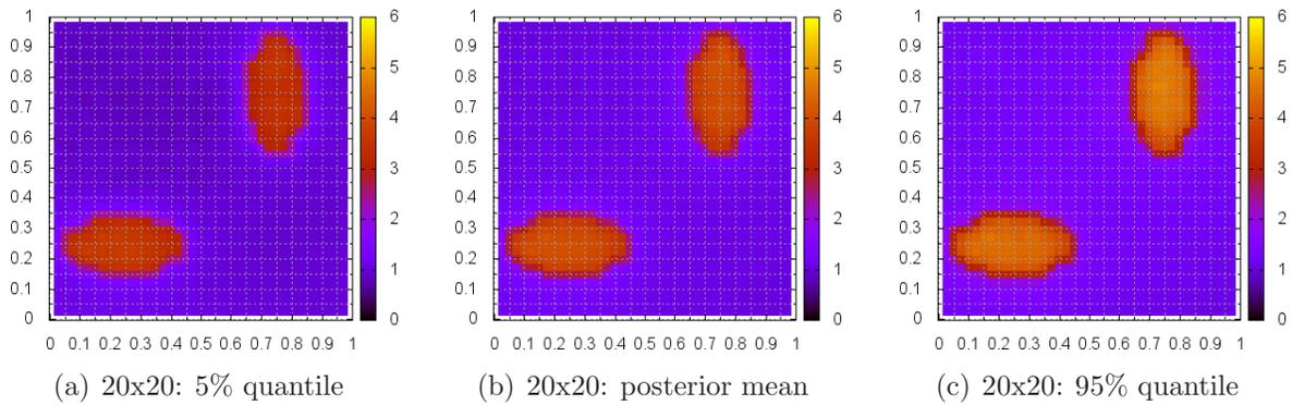
**Figure 4.** Example 1: Posterior statistics of the elastic modulus distribution for noiseless data.
