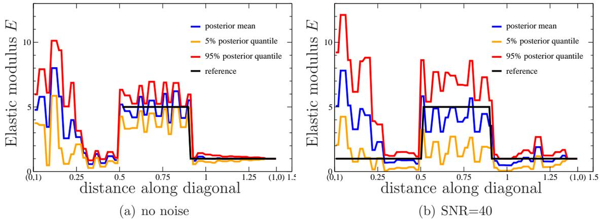
**Figure 10.** Example 2: Posterior statistics of the elastic modulus distribution along the diagonal from (0, 1) to (1, 0)
