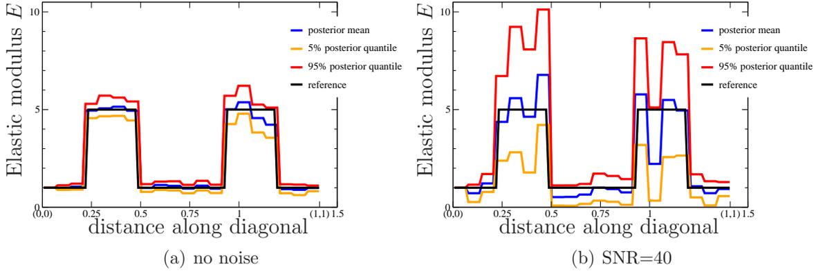
**Figure 6.** Example 1: Posterior statistics of the elastic modulus distribution along the diagonal from (0,0) to (1,1).
