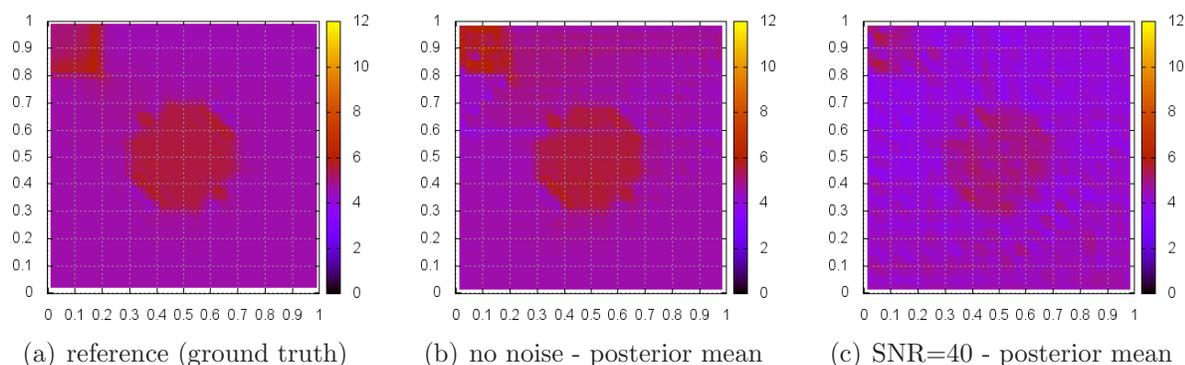
**Figure 11.** Example 2: Comparison of pressure's spatial distribution with the posterior means obtained when data have no noise and for SNR=40dB.
