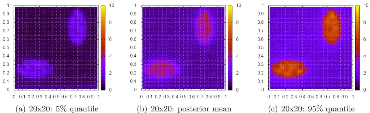
**Figure 5.** Example 1: Posterior statistics of the elastic modulus distribution for noisy data with  $SNR=40dB$ .
