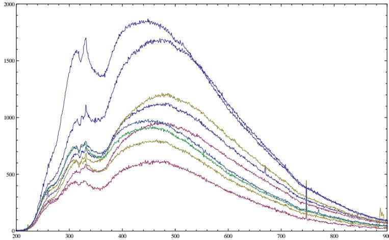
Figure 5: raw dark current subtracted spectrum of SBSL of sample selected for calibration of spectrometer
