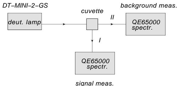
Figure 8: Configuration for test of calibration by measurements of emission spectra of D-L,L-Tryptophan
