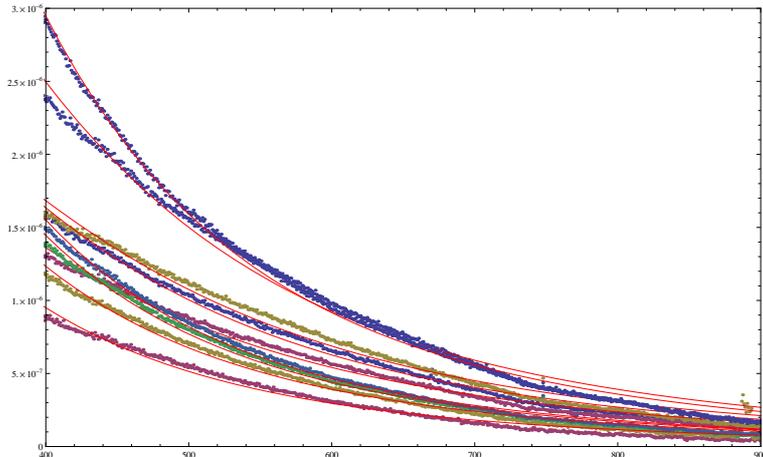
Figure 6: Same sample as in Fig. 5 spectra corrected by absolute irradiance calibration of spectrometer in 400 - 900 nm wavelength region. Results of black-body fits are included there (red lines).
