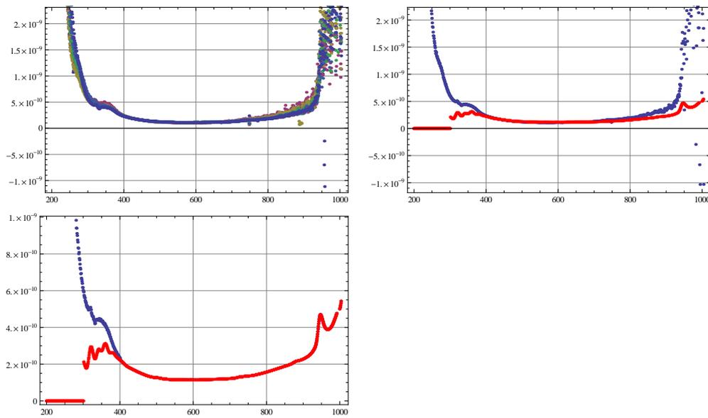
Figure 7: Upper left - derived calibration functions from selected SBSL sample, upper right - average calibration function (from selected) compared with original calibration function based on lamp LS-1-CAL, bottom left - combined calibration function.
