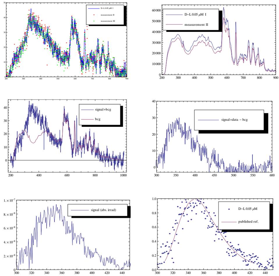
Figure 9: Emission spectra study from D-L tryptophan of concentration  $0.05 \mu M$  in water.
