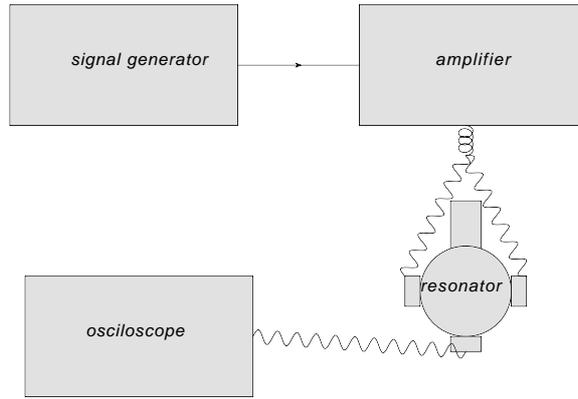
Figure 1: schematic view of apparatus for SBSL
