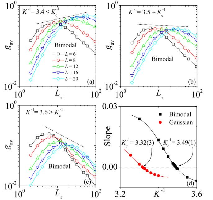
FIG. 1. (a)-(c) Show the Binder cumulant for the bimodal case, as function of  $L_\tau$  for different lattice sizes  $L$  and three temperatures as indicated. (d) Shows for both, the bimodal and the Gaussian cases, the slope of the straight line that intersects the maxima of the Binder ratio,  $g_{\text{av}}^{\text{max}}$ , against  $K^{-1}$ .
