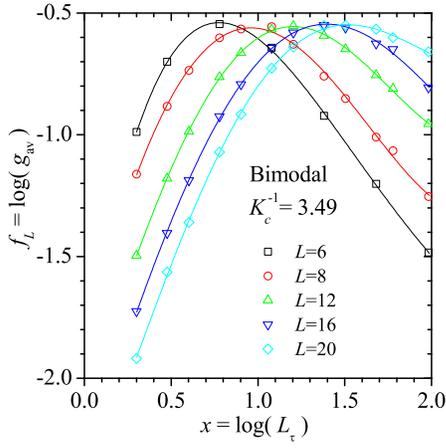
FIG. 5. (Color online) The logarithm of the Binder cumulant versus the logarithm of  $L_\tau$ , for the bimodal case and for different lattice sizes  $L$  as indicated. Open points correspond to simulation results while continuous lines are fits made with a fourth-order polynomial.
