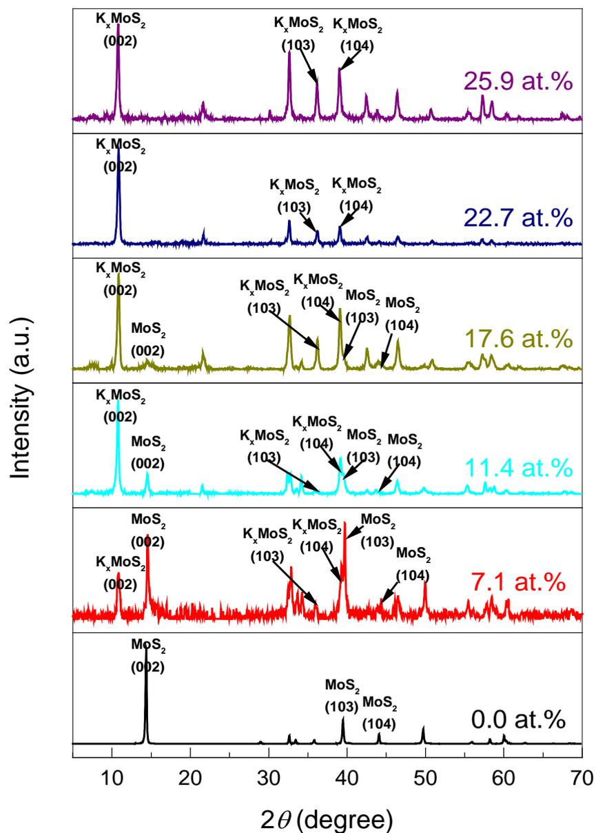
**Supplementary Figure S3 | Labelling of XRD peaks.** Examples of XRD spectra for pristine (bottom curve) and intercalated  $\text{MoS}_2$ , at different average K concentrations. Labels are shown for all main peaks. Average K concentrations,  $c$ , are shown by numbers above each spectrum. The shifts of (002), (103) and (104) peaks to lower  $2\theta$  indicate the expansion of the crystal lattice along the  $c$ -axis upon intercalation.
