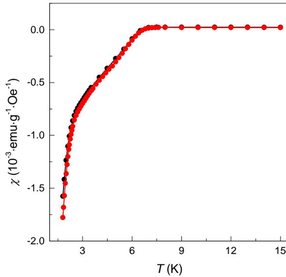
**Supplementary Figure S7 | Reproducibility of the superconducting response and stability of the superconducting phases.** Shown is the temperature-dependent dc magnetic susceptibility,  $\chi = M/H$ , for an intercalated sample with  $c \approx 23$  at.% measured immediately after intercalation (black symbols) and after one month in the glove box (red symbols). Here  $M$  is the magnetic moment measured in ZFC mode at  $H = 10$  Oe.
