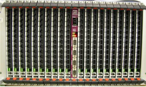
Fig. 3 Service Board and PDM Crate without cables connection.
