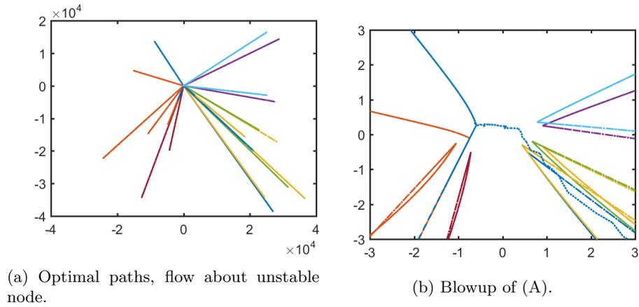
Figure 5: (A) Optimally controlled glider velocities for flow about unstable node. Solid lines are optimally controlled, dashed lines have no control, and dotted lines have random control. (B) Same as in (A) but with axes rescaled to give better picture of uncontrolled and randomly controlled paths.
