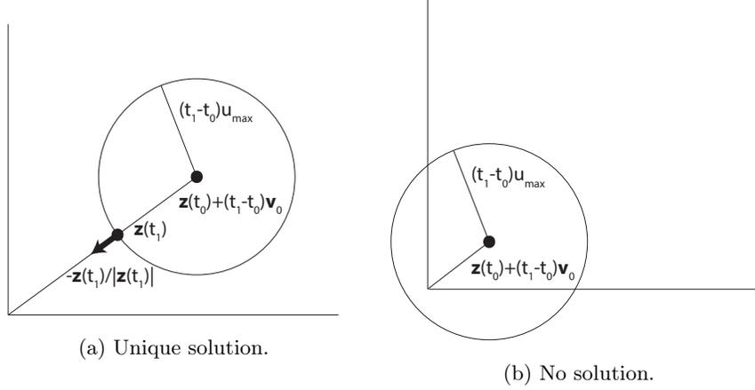
Figure 1: (A) Illustration of unique solution to condition 29 when  $\|z(t_0) + (t_1 - t_0)v_0\| > (t_1 - t_0)u_{\max}$ . (B) Illustration that no solution exists when  $\|z(t_0) + (t_1 - t_0)v_0\| < (t_1 - t_0)u_{\max}$ .
