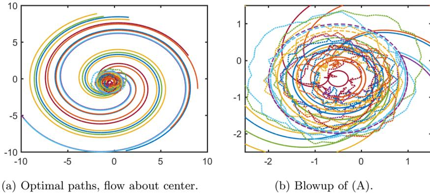
Figure 3: (A) Optimally controlled glider velocities for flow about center. Solid lines are optimally controlled, dashed lines have no control, and dotted lines have random control. (B) Same as in (A) but with axes rescaled to give better picture of uncontrolled and randomly controlled paths.
